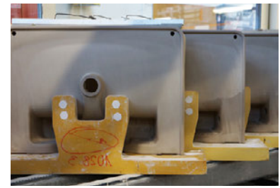
PRODUCTION OF SAPHIRKERAMIK WITH THE CASTING TECHNOLOGY INVENTED BY LAUFEN
