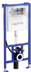
LIS H894666 Installation system LIS CW2 with cistern for wall-hung WC and shower toilet, dual flush 4.5/3L (adjustable to 6/3L)
