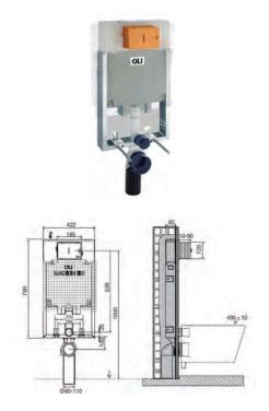
OLI80 is ideal for wall-hung toilets and is suitable for application in masonry walls or solid-walls that are bricked lined. this cistern is compatible with all wall-hung pans Dual flush cistern Technical features include: - Structure: Metal, galvanized, corrosion-resistant- 10 Year guarantee (If the product is not correctly installed the guarantee is not valid).
